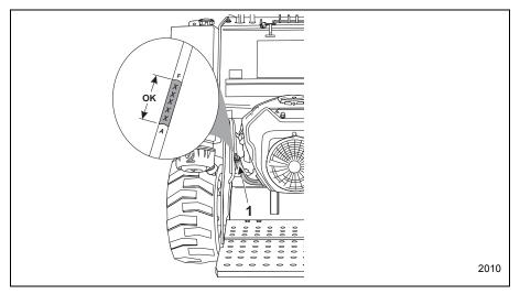
Figure 4-2 Oil Level Check
